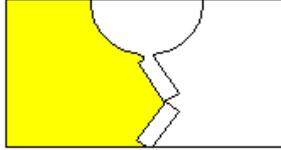
When metal hits this very thin column of investment material (which is the tiny hole you have created for drilling of stone seat) it breaks!
